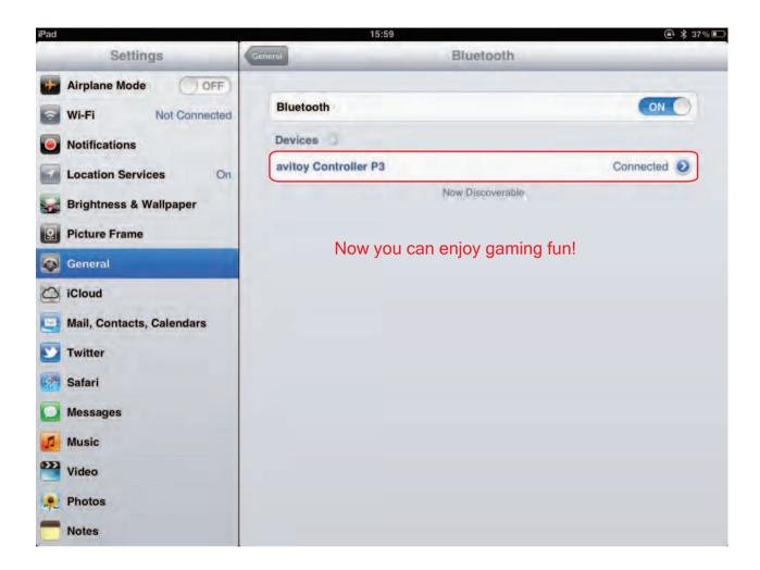
When the controller is connected to the tablet, the Link indicator will stay on, and "connected" will also be shown on the tablet screen just behind "avitoy controller P3". Then when you press the buttons on the controller, the Action indicator will flash.
